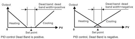
Figure B: Output Operation during dual loop control
