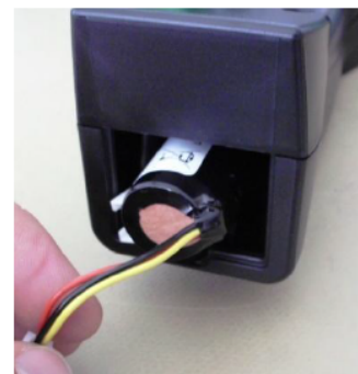
Carefully pull out the battery
