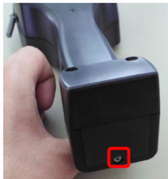
Removing the battery cover
