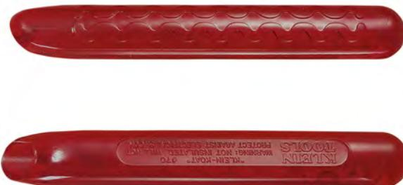
These Tenite-plastic grips handles provide comfort and resist slipping. Use hot tap water to fit these to an existing pair of 8-Inch (203 mm) to 9-Inch (229 mm) pliers.
