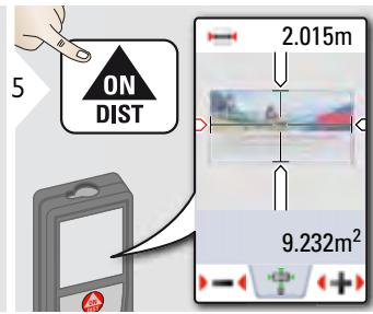
Select arrows with the cursor keys or by tapping on the display and adjust with softkeys. Corresponding area is calculated.
