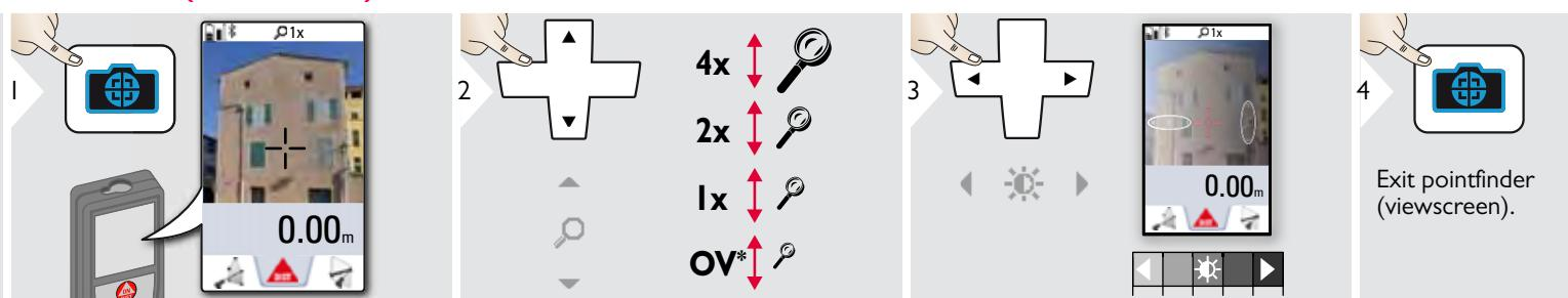
**i** This is a great help for outdoor measuring. The integrated pointfinder (viewscreen) shows the target on the display. The device measures in the middle of the cross hair, even if the laser dot is not visible.
