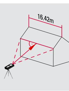
**It is absolutely necessary to aim with the laser perpendicular to the object.**
