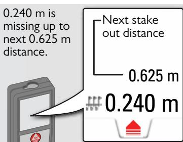
**i** When approaching a stake out point to less than 0.1 m the instrument starts to beep. The function can be stopped by pressing the CLEAR/OFF button.
