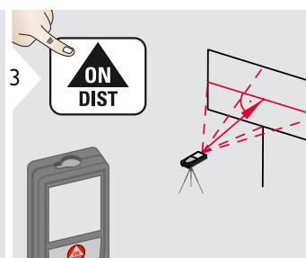
**Aim perpendicular to the horizontal center line of the area. This area must be perfectly flat on the vertical plane.**
