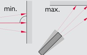
Used to measure room diagonals (maximum values) or horizontal distance (minimum values)
