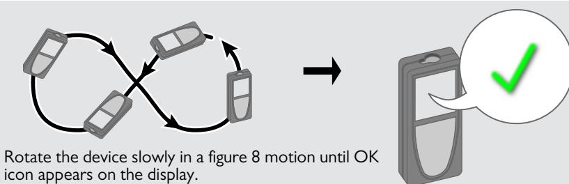
Rotate the device slowly in a figure 8 motion until OK icon appears on the display.
