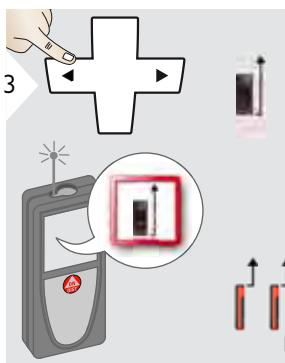
Distance is measured from the rear of the device (standard setting).
