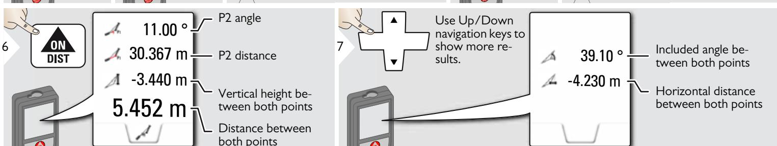
**i** Indirect distance measuring between 2 points with additional results. Ideal for applications such as length and slope of roof, height of chimneys,....
