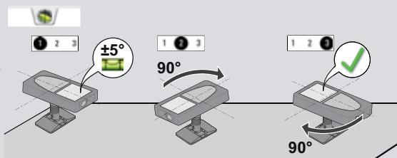
Rotate the device two times clockwise  $90^\circ$ . Follow the instructions on the display. Levelling is finished when OK icon appears on the display.
