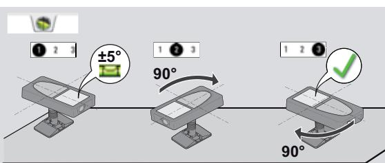
Rotate the device two times clockwise  $90^\circ$ . Follow the instructions on the display. Levelling is finished when OK icon appears on the display.
