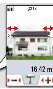
Select arrows with the cursor keys or by tapping on the display and adjust with softkeys. Corresponding width is calculated.
