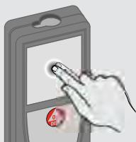
Tap on the display to open an on-screen button or to make a selection. Tapping on the icon in the middle of the bottom line activates the distance measurement or triggers the camera.
