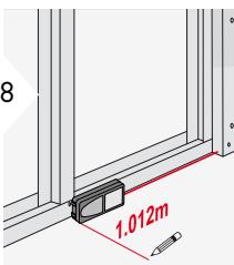
Move device slowly along the stake-out line. The distance to the next stake out point is displayed.
