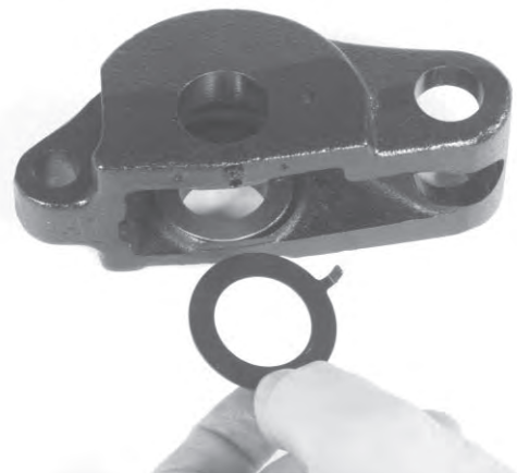
Figure 18 – Inserting Tabbed Thrust Washer
