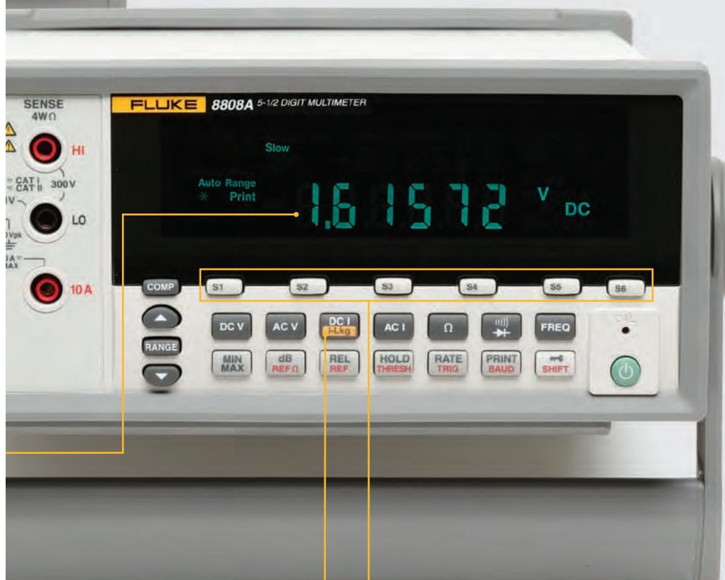
i-Lkg function adds two additional hi-impedance ranges for sensitive low current measurements
