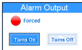
Figure 22 – Alarm output with forcing in on status
