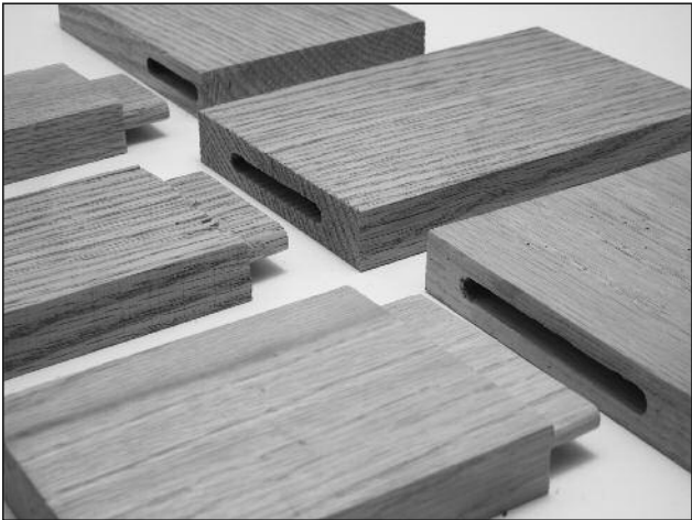
Sample Mortise & Tenon Joints
