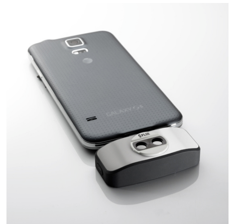
Figure 31.3 2015: FLIR One, an accessory to iPhone and Android mobile phones. Weight: 90 g (3.2 oz.).
