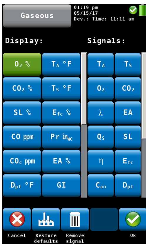
Fig. 36: Configuration of the readings segment.
