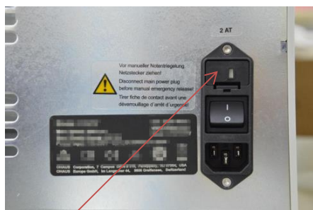
Fuse drawer with fuse 4 AT
