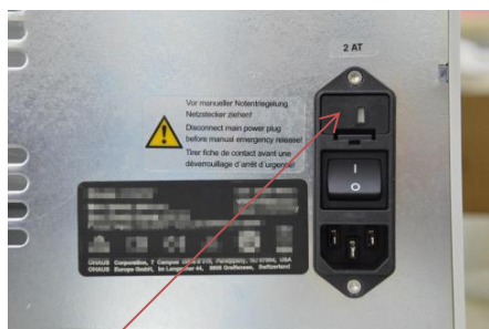
Fuse drawer with fuse 4 AT
