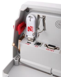
Interface connections on back of Terminal.
