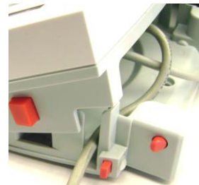
Interface connections on back of Terminal.
