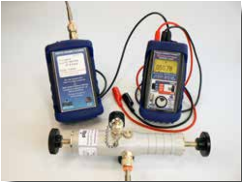
PIE 830 with Pressure Module, Pressure/Vacuum Pump & Hose
