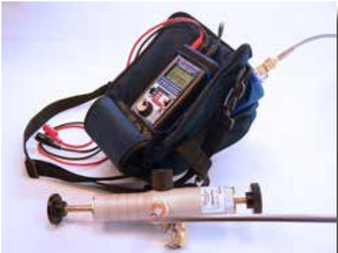
PIE 830 with Pressure Module, Pressure/Vacuum Pump & Hose
