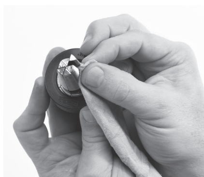
Figure 10 – Cleaning The Expander Head
