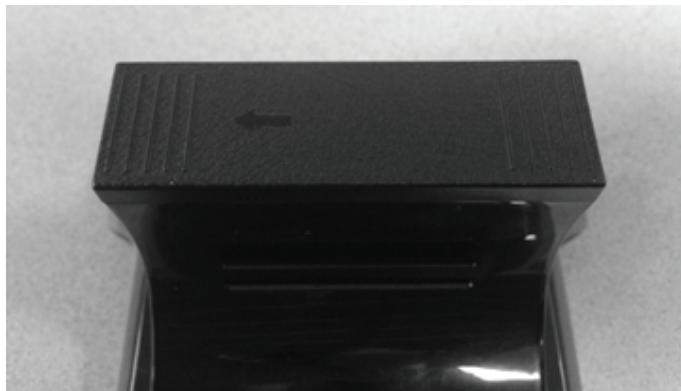
Slide battery cover to the left (See arrow on cover) to remove the battery cover
