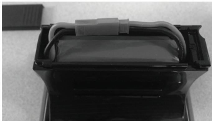
Connect them, by inserting the battery connector into the battery terminal connector of the product. Replace cover once battery leads are connected.
