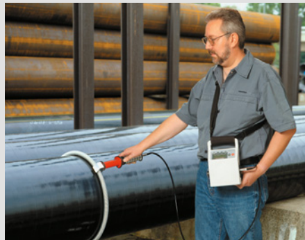
Porosity detection on pipelines
