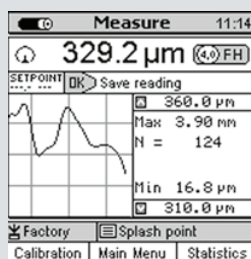
Measuring Value combined with Real-Time Trend Diagram
