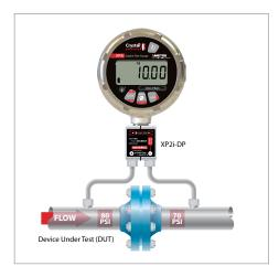
The pressure measurement accuracy of the gauge in this example is a combination of the standard accuracy statement and the static line pressure effect. The 10 psid pressure, when compared to the 100 psi full scale product used, will require the 0 to 20% of Full Scale, ± (0.02% of Full Scale) accuracy statement. The static line pressure effect relates to the lowest test pressure applied in the test, or in this case 70 psi. The pressure measurement accuracy for this test condition is as follows:
