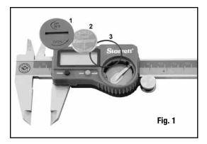
First, unscrew and remove the battery cover (1) by turning it to the left 1/4 turn. Remove the old battery. Next, position the rubber "O" ring (3) correctly in the bottom of the battery compartment before inserting the new battery (2) negative side (-) down. Then, re-install the battery cover (1) and lock it into position by giving it a 1/4 turn to the right.
