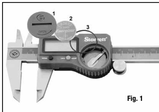
First, unscrew and remove the battery cover (1) by turning it to the left  $\frac{1}{4}$  turn. Remove the old battery. Next, position the rubber "O" ring (3) correctly in the bottom of the battery compartment before inserting the new battery (2) negative side (-) down. Then, re-install the battery cover (1) and lock it into position by giving it a  $\frac{1}{4}$  turn to the right.
