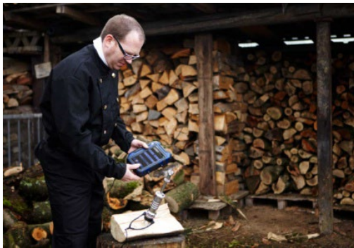
Fig. 40: Wood moisture measurement with Probe Wöhler HBF 420.
