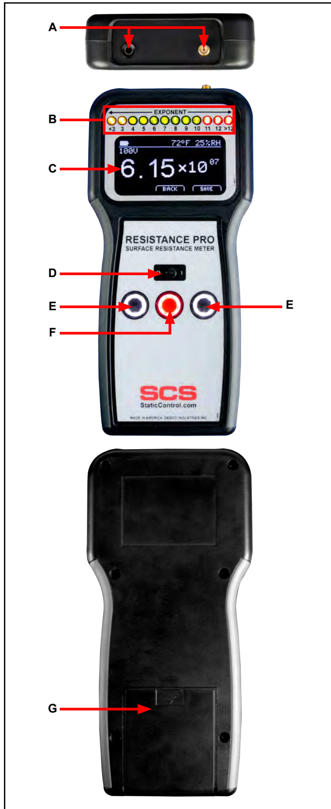
Figure 4. Resistance Pro Meter features and components
