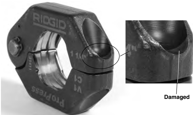
Figure 13 – Damaged Ring Pocket
