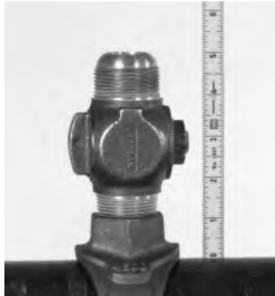
Figure 8 – Measuring valve standoff distance
