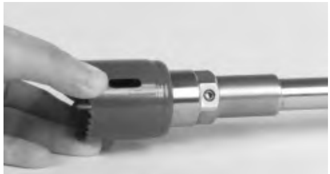
Figure 3a – Installation of large hole saw adapter
