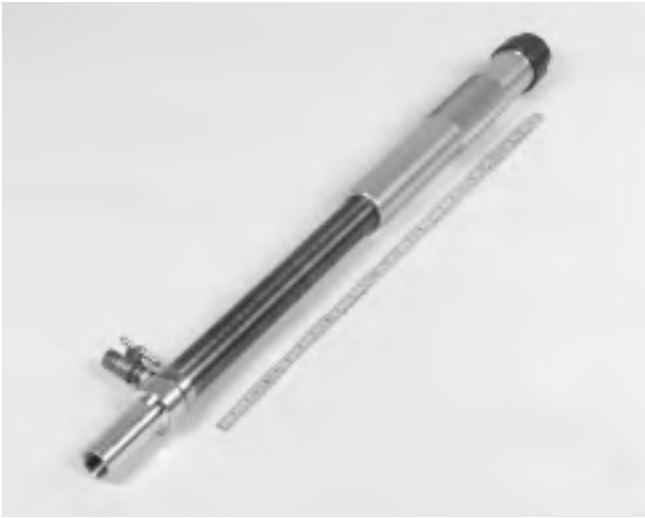
Figure 7 – Measuring full stroke distance
