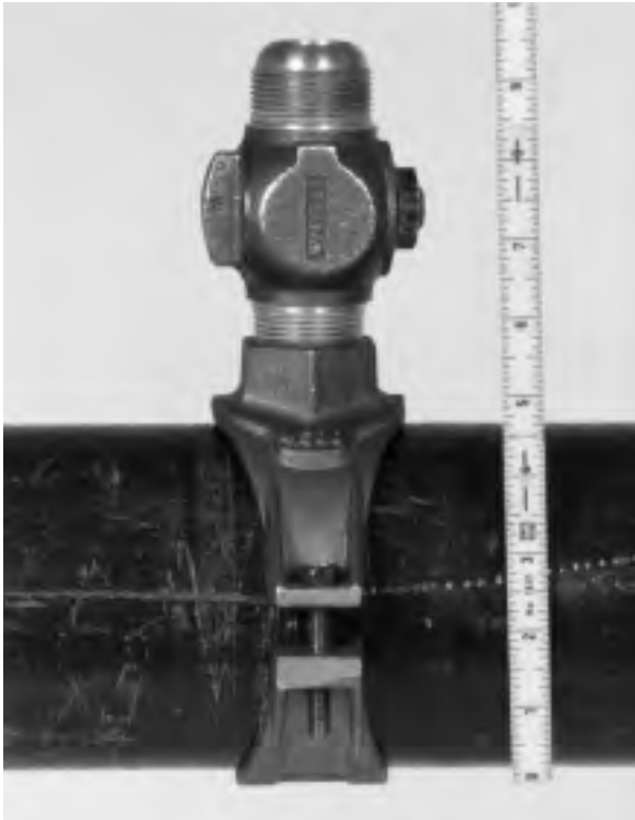
Figure 10 – Measuring maximum stroke
