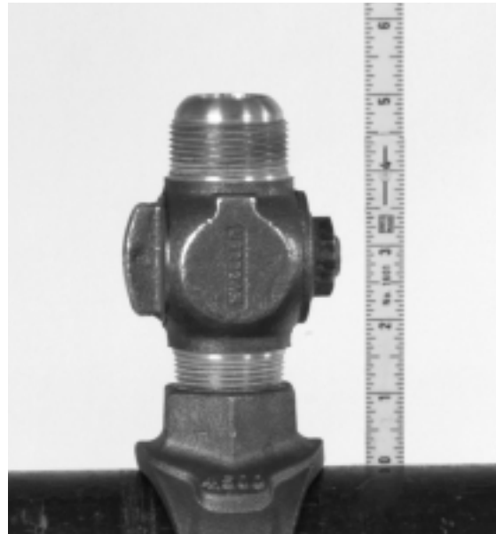
Figure 8 – Measuring valve standoff distance
