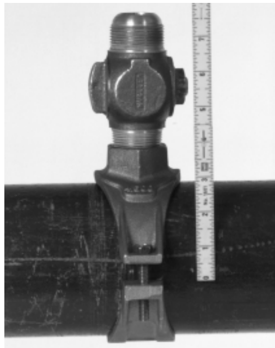
Figure 9 – Measuring valve standoff distance
