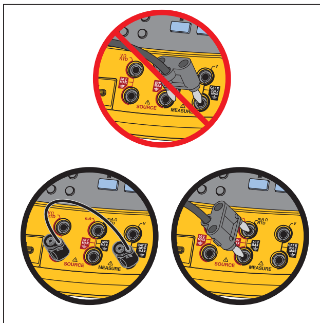
Figure 16. Correct Jumper Use
