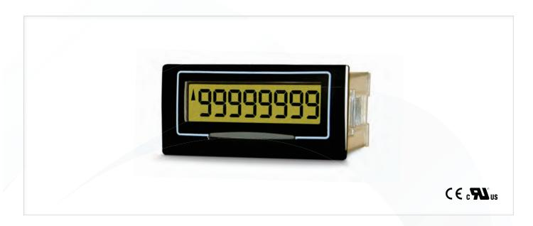
8-digit liquid crystal display timer, self-powered with a 10-year battery life. A compact LCD timer designed for many applications, screw terminals ensure fast wiring. Features include backlighting (external 5VDC supply required), 4 timing modes, timing direction indication and 9mm high digits. High Voltage (HV) version accepts input voltages of 5-110VDC or 10-240VAC.
