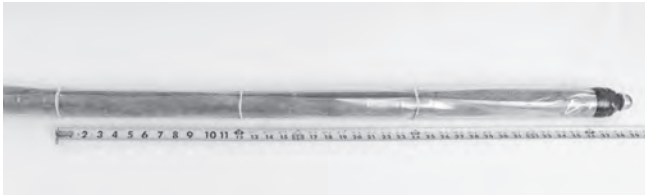
Figure 16 – Elastic Band Placement On Packer Sleeve (Every 12")
