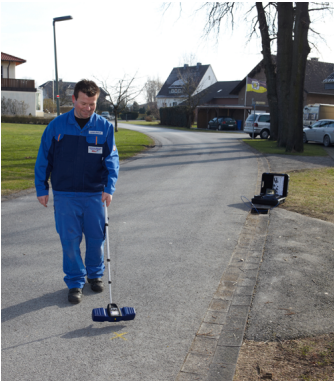
The Wohler VIS 350 precisely locates radio signals transmitted by the camera head through concrete and asphalt to save time and money in repairs.
