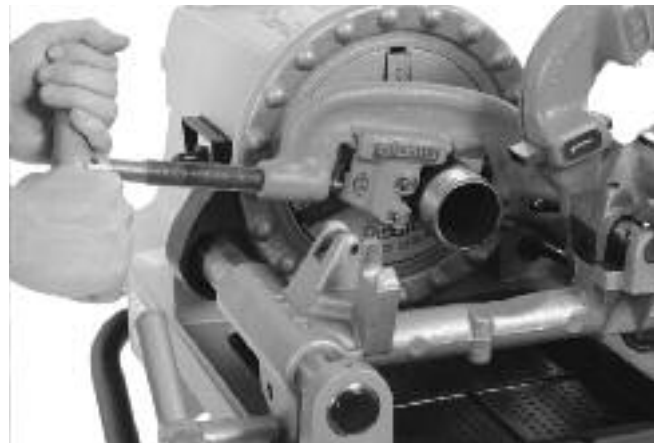
Figure 22 – Cutting Pipe with Cutter
