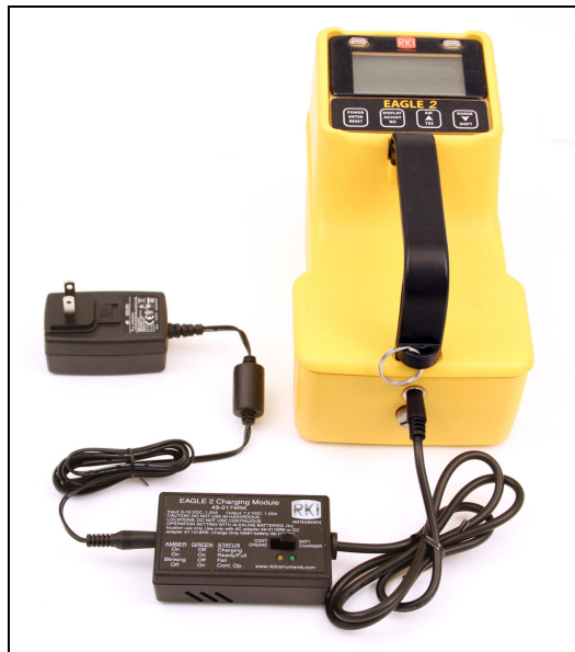
Figure 17: Connecting a Charger to the EAGLE 2
