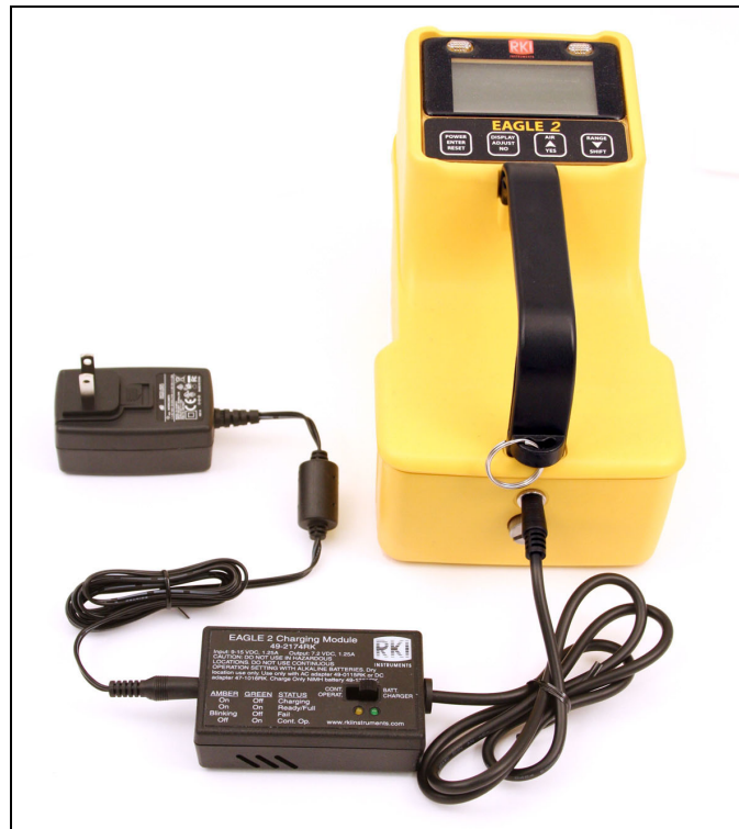
Figure 20: Connecting the Charger to the EAGLE 2
