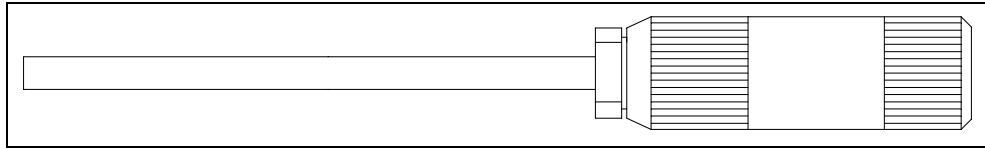
Figure 13: 10 Inch Probe with Dust Filter
