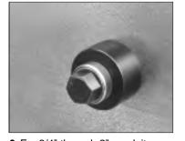
6 For 3/4" through 2" conduit sized holes use 304AVBB 3/4" draw stud. Place selected size die on draw stud. Insert draw stud in 3/4" or larger pilot hole.\* Thread same size punch on the draw stud with the cutting edge toward the material being punched.
