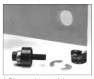
8 Disassemble punch by turning draw stud counter-clockwise while holding punch. Tip die and drop out split slugs.
