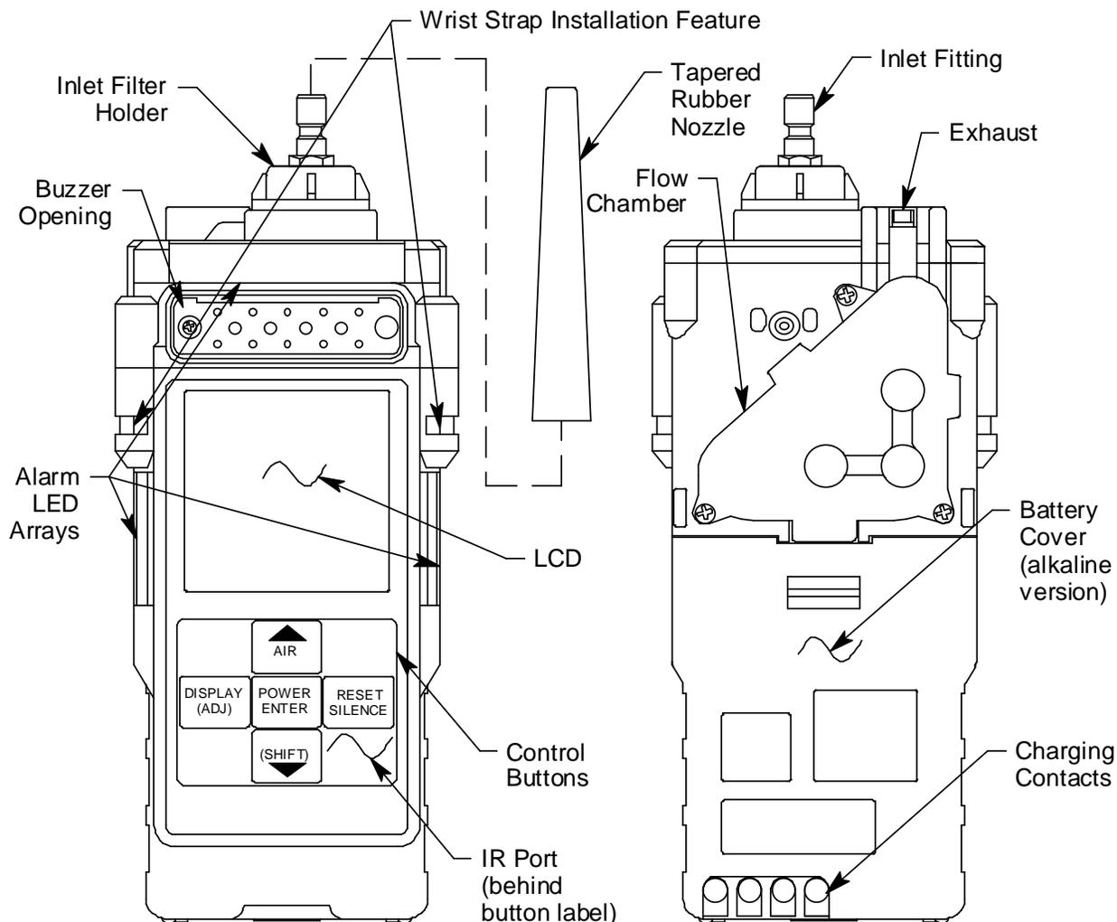
Figure 1: Components of the GX-2012, Front & Back
