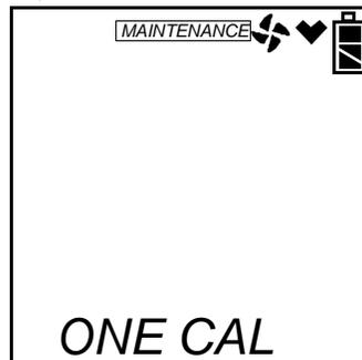
6. Press and release the POWER ENTER button to display the single calibration menu. The %LEL sensor will be displayed first.
