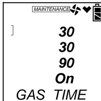
3. To update the GAS TIME setting, with the cursor next to the gas time and with GAS TIME displayed along the bottom of the screen, press POWER ENTER. The factory setting is 30 seconds. The value will begin to flash. Use the AIR▲ or (SHIFT)▼ buttons to select a new gas time. The GAS TIME is the amount of time that the instrument is exposed to gas during a bump test. The time increments are 30, 45, 60, and 90 seconds. Once a value is selected, press and release the POWER ENTER
