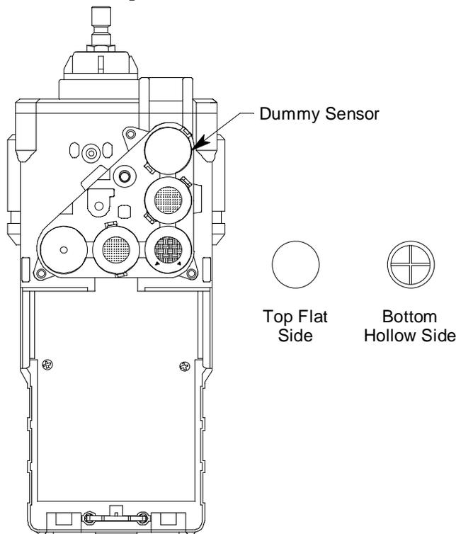
**Figure 3: Dummy Sensor**
