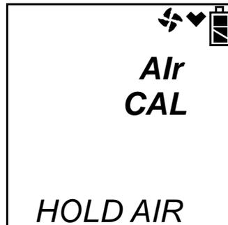
4. Continue to hold the AIR▲ button until the display prompts you to release the AIR▲ button. The GX-2012 will set the fresh air reading for the combustible channel. Once the fresh air adjustment has finished, start up is complete and the unit is ready for leak testing.
