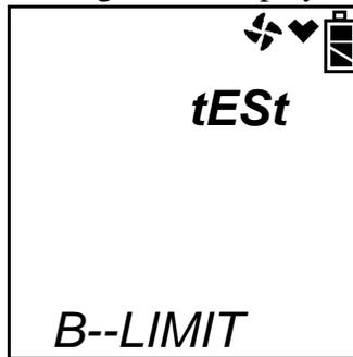
The alarm LED's and buzzer will pulse several times. After this, press the RESET SILENCE button until you hear a beep to continue.
