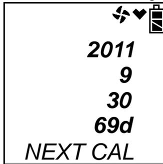
7. If **BP RMNDR** is turned on (factory setting is OFF), the screen that appears next depends on how **BP EXPRD** is set in the Maintenance Mode Menu ((pg. 119)).
