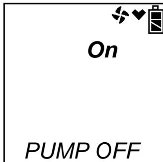
In this screen, press POWER ENTER to turn the pump off. The fan in the upper right corner of the screen will disappear. Once the pump is off, you cannot exit this screen and return to normal operation or continue in Display Mode until you turn the pump back on. To turn the pump back on and continue in Display Mode or return to Normal Operation, press the POWER ENTER button again.
