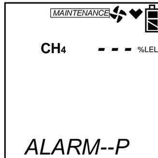
2. You may then select a channel. Use the AIR▲ or (SHIFT)▼ buttons to select a channel. The combustible gas channel is shown for example.
