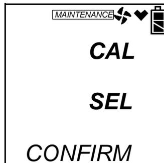
2. Use the **AIR▲** or **(SHIFT)▼** button to display the desired setting along the bottom of the screen.
