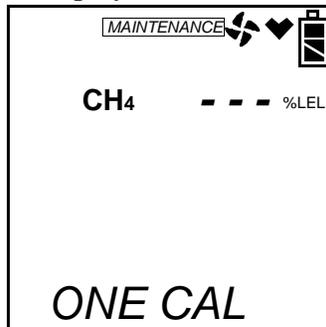
3. Use the AIR▲ or (SHIFT)▼ button to display the sensor you want to calibrate (in this example the combustible gas % LEL sensor). If you have a 5 sensor unit, the % vol sensor will be one of the choices. It is shown below.
