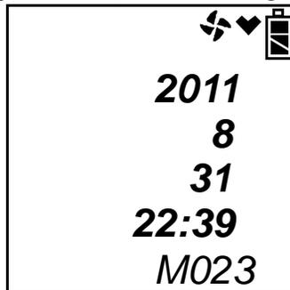
This screen indicates the year, month, day, and time that the most recent snap log was taken. The number along the bottom of the screen indicates the snap log ID number. The first snap log that is taken is given an ID of M001. The next snap log ID is M002. The ID number increases sequentially with each set of snap log data. Use the AIR▲ and (SHIFT)▼ buttons to scroll through different snap log IDs and view what time they were taken.
