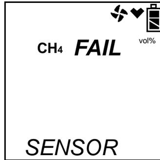
If one of the combustible sensors, LEL or % volume, fails, it is not possible to enter Bar Hole Mode. Press and release the RESET SILENCE button to acknowledge the failure and return to the Mode Select Screen. Replace the failed sensor as soon as possible.
