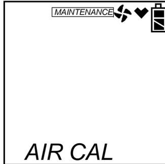
3. Press and release the POWER ENTER button to enter **AIR CAL**. The current gas readings are displayed.
