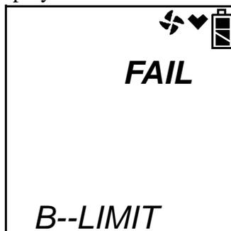
The GX-2012 cannot be used until a bump test has been performed by selecting **BUMP** in the Maintenance Mode menu. See “Performing a Bump Test” on page 102 for bump testing instructions.
