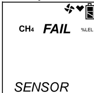
If the catalytic LEL sensor fails, it is not possible to enter Leak Check Mode. Press and release the RESET SILENCE button twice to acknowledge the failure and return to the Mode Select Screen. Replace the failed sensor as soon as possible.
