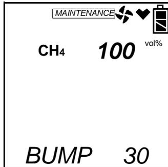
**NOTE:** If you wish to change any of the bump test gas values, you must exit the **BUMP** menu item and enter the **AUTO CAL** menu item. See steps 8 through 15 in “Calibrating Using Auto Calibration” on page 97 for instructions to change the gas values.
