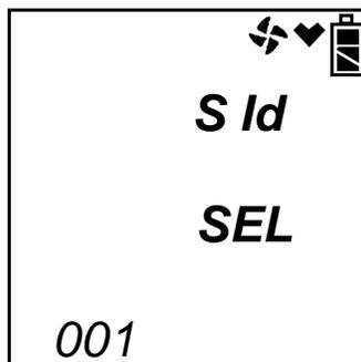
Use the AIR▲ and (SHIFT)▼ buttons to scroll to the desired station ID and press and release POWER ENTER. The unit will return to the Bar Hole Measuring Screen.
