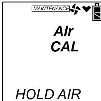
5. When the unit tells you to release the AIR▲ button, release it. The unit will count down from 8 as it performs the fresh air adjust.
