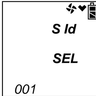
2. Use the (SHIFT)▼ and AIR▲ buttons to scroll to the desired station ID, then press and release the POWER ENTER button to continue to the Base Reading Screen. To return to the Station ID Select Screen without taking a base reading, press and release the RESET SILENCE button.
