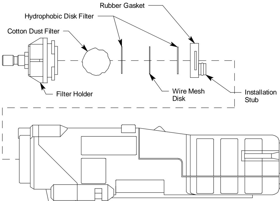
**Figure 29: Changing the Filters & Wire Mesh Disk**
