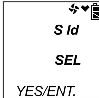
**NOTE:** As shipped from the factory, the station ID on this screen is shown as ----- until you enter this screen and select a station ID.
