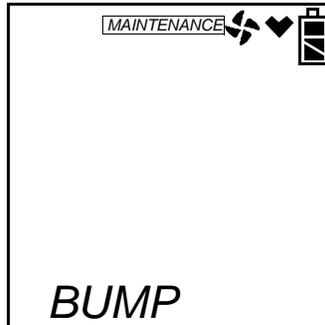
9. Press and release the POWER ENTER button to display the bump test gas values.
