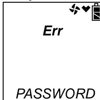
To return to normal operation, press and release the RESET SILENCE button. You may then try to reenter Calibration Mode.
