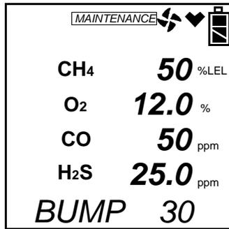
7. Use the AIR▲ or (SHIFT)▼ buttons to see the % volume combustible gas bump test value.
