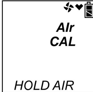
4. Continue to hold the AIR▲ button until the display prompts you to release the AIR▲ button. The GX-2012 will count down from 8 on an autoranging combustible gas channel as it sets the fresh air reading for all channels. Once the countdown has finished, start up is complete and the unit is ready for monitoring.
