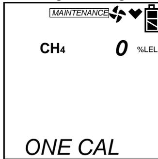
5. Connect the tubing from the demand flow regulator to the rigid tube on the probe. Allow the calibration gas to flow for one minute.
