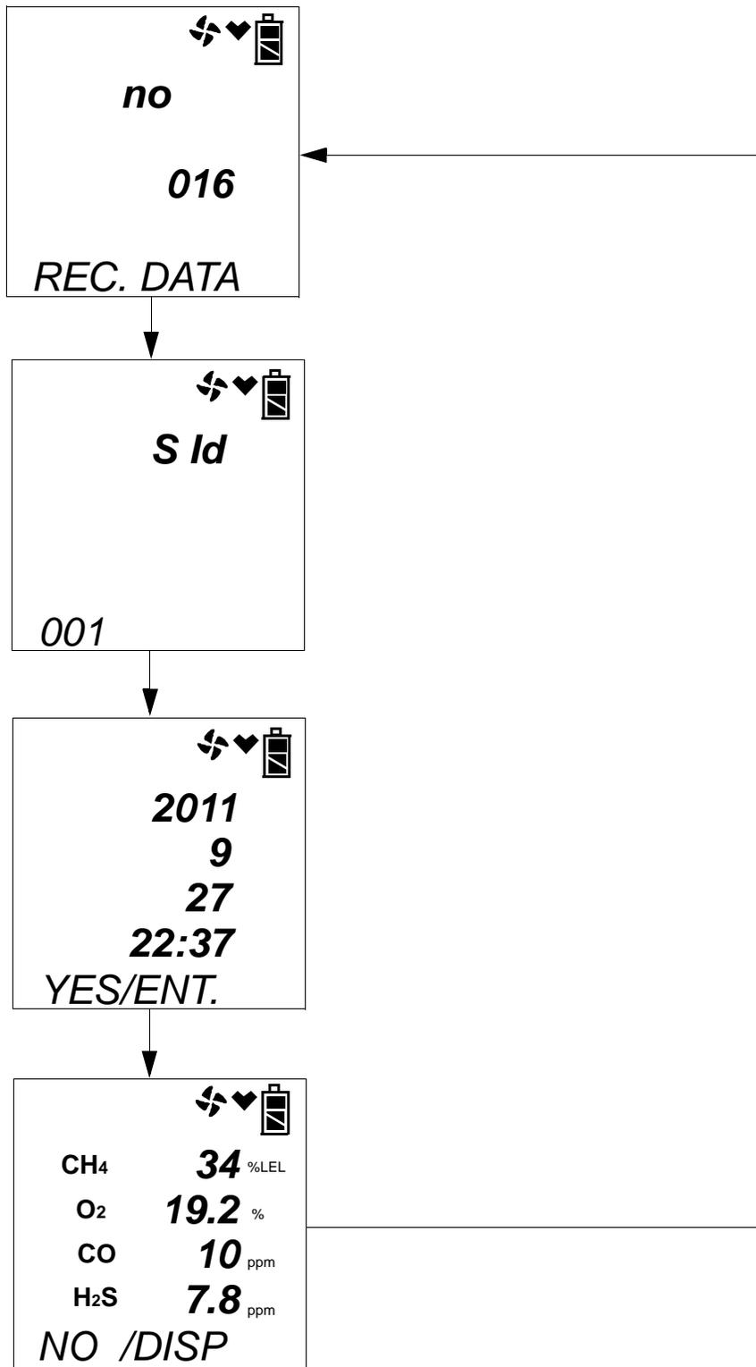
The first screen displays what snap log ID will be given to this particular set of data. This ID number increases sequentially with each set of snap log data taken. The second screen displays what Station ID will be associated with this snap log. The third screen displays the year, month, day, and time of the snap log, and that you should press the POWER ENTER button to save a set of snap log data. The fourth screen
