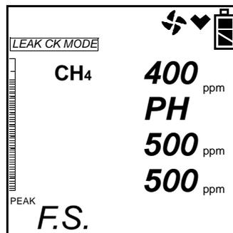
The current methane reading is displayed on the first line. The “PH” shown on the second line indicates that the GX-2012 is in Peak Hold Mode. The peak methane reading is displayed on the third line. The full scale value is displayed on the fourth line.
