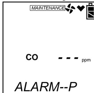
14. Use the AIR▲ or (SHIFT)▼ buttons to select the H<sub>2</sub>S channel and press POWER ENTER. Adjust the values for the warning and alarm settings using the procedure in step 4 through step 7. When you press POWER ENTER after selecting the alarm value, you will then be prompted to select the STEL value as you were with the CO channel.
