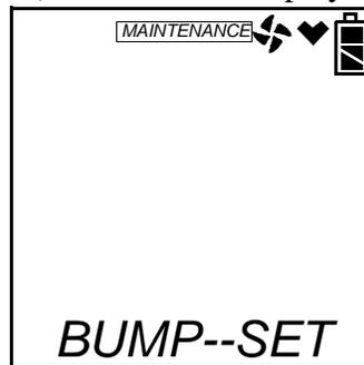
2. Press and release the POWER ENTER button. The values displayed are for GAS TIME, CHECK (bump test tolerance), CAL TIME, and AUTO CAL. The cursor on the left of the screen shows which setting is associated with the parameter shown at the bottom of the screen. Use the AIR▲ or (SHIFT)▼ buttons to scroll up or down along the list.
