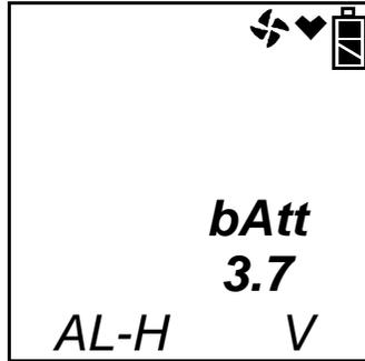
AL -- H indicates latching (hold) alarms and AL -- A indicates self-resetting (automatic) alarms. The number shown indicates the voltage of the batteries. If the unit is powered by alkaline (dry cell) batteries, a “D” will appear before the “V” in the lower right corner.
