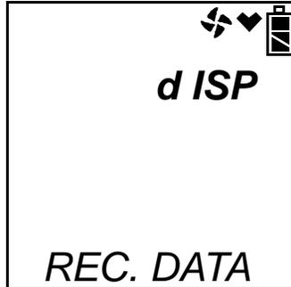
2. Press and release the POWER ENTER button. If no snap logs have been performed, the following screen will appear.
