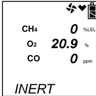
3. Since the oxygen concentration in fresh air is above both oxygen alarm points, the GX-2012 will go into alarm if turned on in a fresh air environment.
