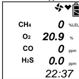
The concentrations of the target gases are displayed along with the time and battery charge level. The heart symbol displayed just to the left of the battery charge level flashes while the instrument is functioning properly. If it disappears or is steadily on, the unit is experiencing a microprocessor error. The fan symbol just to the left of the heart symbol spins while the pump is operating.
