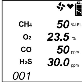
The gas readings that were taken during the snap log are displayed and the Station ID that was in use during the snap log is displayed along the bottom of the screen. You can use the AIR▲ and (SHIFT)▼ buttons to scroll through the different snap logs. The gas readings and station ID will change but the snap log ID is not visible from this screen. To scroll through the data by viewing the snap log ID number, press and release POWER ENTER.
