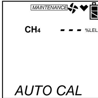
6. Use the AIR▲ and (SHIFT)▼ buttons to scroll through the sensors and select the sensor whose calibration gas value you want to adjust.
