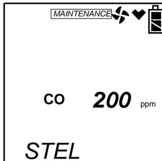
12. Use the AIR▲ or (SHIFT)▼ buttons to change the setting and press POWER ENTER when finished to save the setting. You will then be asked to enter a TWA value.
