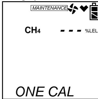
7. Use the AIR▲ or (SHIFT)▼ button to display the sensor you want to calibrate (in this example the combustible gas % LEL sensor). If you have a 5 sensor unit, the %vol sensor will be one of the choices. It is shown below.
