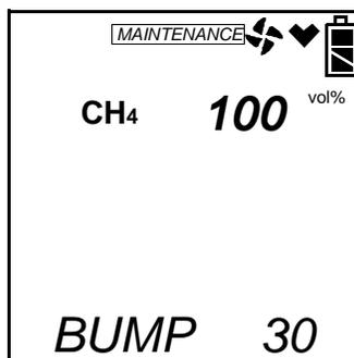
11. A bump test may be performed on the standard 4 sensors or on the % volume combustible sensor. Use the AIR▲ or (SHIFT)▼ buttons to display the screen for the sensor(s) you wish to bump test.
