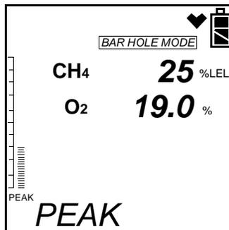
7. If a high concentration of methane is encountered, a fresh air purge can be performed to purge the hose, probe and GX-2012 of gas before the next bar hole test. To perform a purge, do the following:
