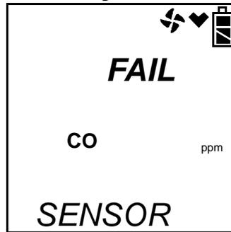
If you wish to continue, press and release the RESET SILENCE button to acknowledge the failure. The gas reading for the failed sensor will be replaced by “---”. Replace the failed sensor as soon as possible.
