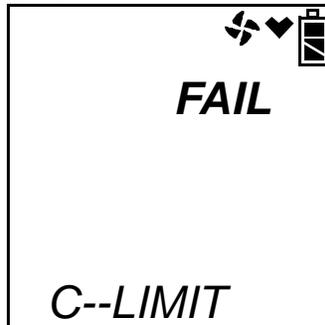
The GX-2012 cannot be used until a calibration has been performed either by selecting **AUTO CAL**, or **ONE CAL** in the Maintenance Mode menu. See "Calibrating Using Auto Calibration" on page 97 or "Calibrating Using Single Calibration" on page 100 for calibration instructions.
