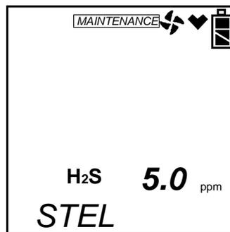
15. Use the AIR▲ or (SHIFT)▼ buttons to change the setting and press POWER ENTER when finished. You will then be asked to enter a TWA value.
