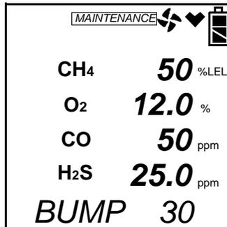
10. Use the AIR▲ or (SHIFT)▼ buttons to see the % volume combustible gas bump test value.
