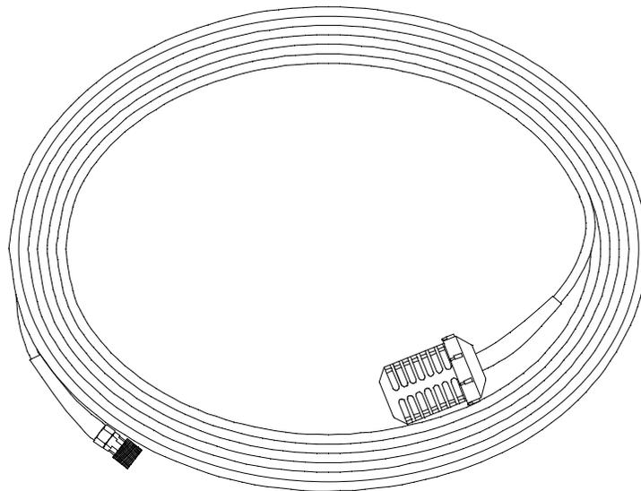
**Figure 15: 8 Meter Hose with Floating Head**
