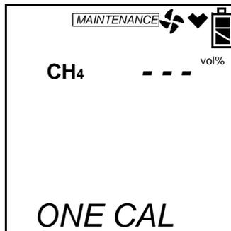
8. Press and release the POWER ENTER button. The single calibration screen displays for the sensor you selected. The gas reading flashes.
