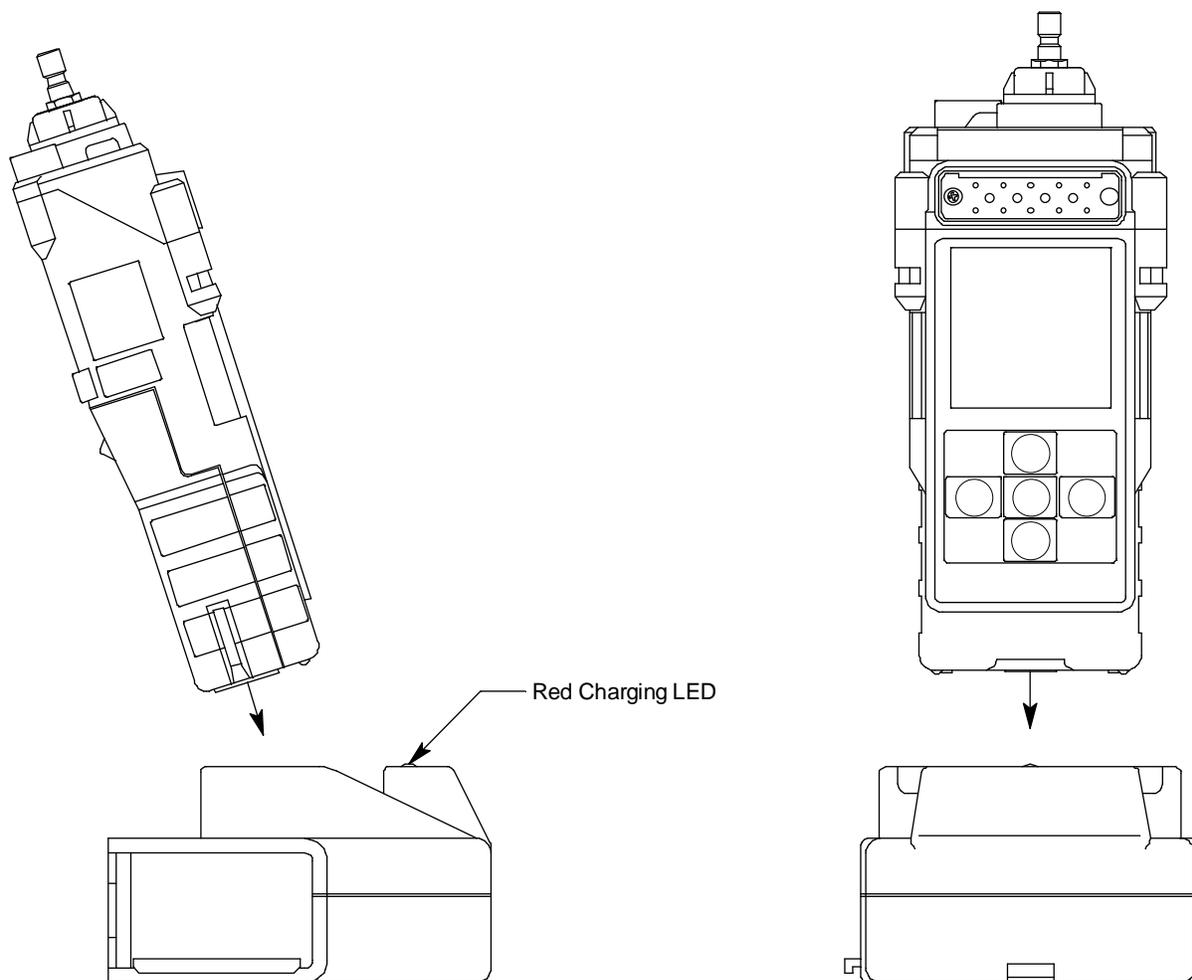
**Figure 23: Putting the GX-2012 into the Charging Station**
