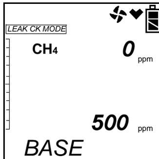
3. In order to get a base, or background, reading, take the instrument a few feet away from where you intend to test. To save the base reading, press and release the POWER ENTER button.
