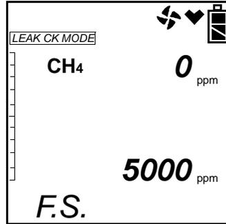
The combustible gas reading is displayed along with the battery charge level.
