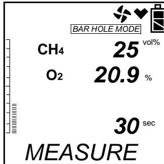
5. After 15 seconds of sampling, if the combustible gas reading is less than 5 % VOL, the combustible gas channel will automatically begin displaying in %LEL.
