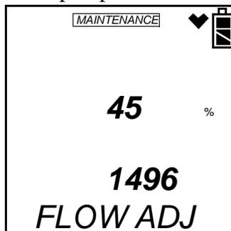
2. Use the AIR▲ or (SHIFT)▼ buttons to get a reading of approximately 1500 on the bottom value. When you have adjusted the value as close as you can, press and release the POWER ENTER button.
