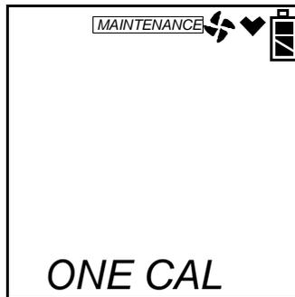
2. Press and release the POWER ENTER button to display the single calibration menu. The %LEL sensor will be displayed first.
