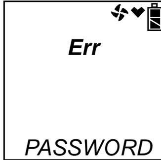
You must turn the unit off and reenter Maintenance Mode using the correct password.
