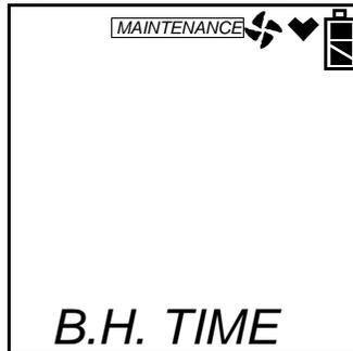
2. Press and release the POWER ENTER button. The screen will indicate the current setting.
