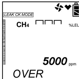
**NOTE:** If a vol% sensor is installed, "OVER" will still appear at the bottom of the screen but the instrument will display the gas reading in % volume.
