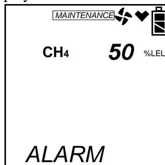
6. Use the AIR▲ or (SHIFT)▼ buttons to change the alarm setting.
