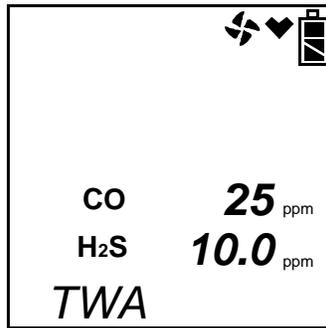
Pressing and releasing POWER ENTER while in a settings screen will cause the instrument to simulate that condition. The buzzer, LEDs, and vibration will activate. Press and release POWER ENTER again to stop the simulated alarm.
