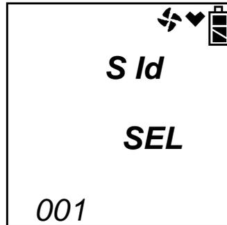
3. Use the (SHIFT)▼ and AIR▲ buttons to scroll to the desired station ID, then press and release the POWER ENTER button to return to the Snap Logging Screen sequence.
