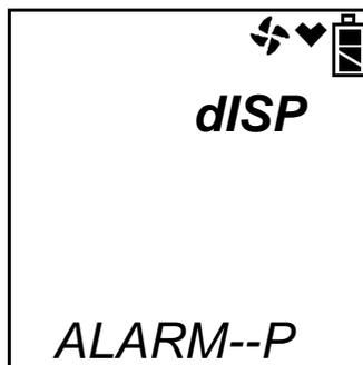
Press the POWER ENTER button to proceed to view the full scale settings. Use the AIR▲ or (SHIFT)▼ buttons to scroll through screens showing the different settings.
