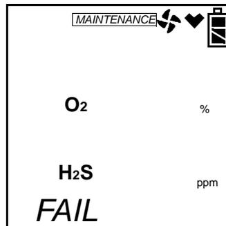
The buzzer and alarm lights activate. Press and release the RESET SILENCE button after the buzzer and lights stop to reset the alarm and return to the calibration menu. Attempt to calibrate again. If the failure continues, investigate the cause. See “Troubleshooting” on page 131.
