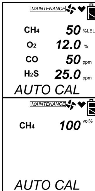
4. The gas concentrations displayed in the calibration values screens must match the gas
