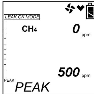
5. Take the instrument to the monitoring area. The instrument will retain and display the highest gas concentration encountered. To save the peak reading, press and release the POWER ENTER button. The reading on the screen (the highest concentration encountered) will be saved.
