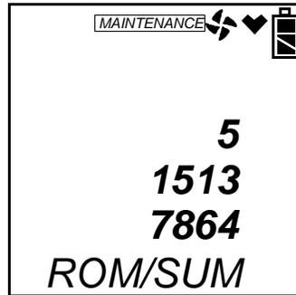
The first two lines display the ROM number. The ROM number indicates the firmware version number. In the above example, the ROM number is 51513. The bottom line displays the SUM number, 7864 in the above example.
