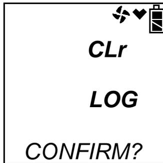
2. To cancel the clear data log and return to the Clear Data Logger Screen in Display Mode, press and release DISPLAY (ADJ).
