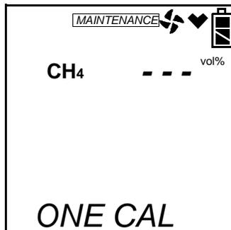
4. Press and release the POWER ENTER button. The single calibration screen displays for the sensor you selected. The gas reading flashes.
