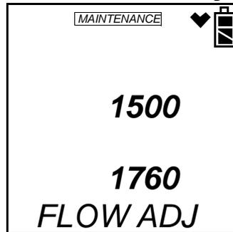
Connect a flow meter to the inlet of the instrument and adjust it to  $0.5 \text{ SCFH} \pm 0.1 \text{ SCFH}$ . This will be the low flow setpoint. You do not need to adjust anything at the instrument. Once the low flow setpoint is set, press and release the POWER ENTER button.
