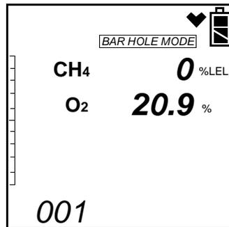
The methane and oxygen channels are displayed along with the battery charge level.
