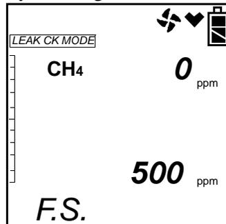
Continue to press and release the DISPLAY (ADJ) button until the desired display range value is displayed.
