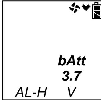
AL -- H indicates latching (hold) alarms and AL -- A indicates self-resetting (automatic) alarms. The number shown indicates the voltage of the batteries. A fully charged lithium ion battery pack will display 3.7 V. If the unit is powered by alkaline (dry cell) batteries, a “D” will appear in front of the “V” in the lower right corner.
