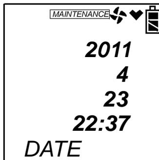
2. Use the AIR▲ or (SHIFT)▼ button to display the desired year.
