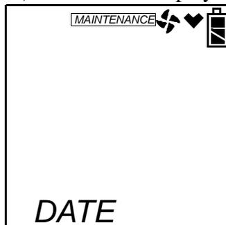
Press and release the POWER ENTER button. The date and time will be displayed with the year flashing.
