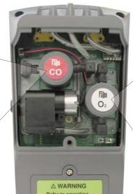
A761S Smart 02 Sensor Pre-calibrated smart 02 sensor
