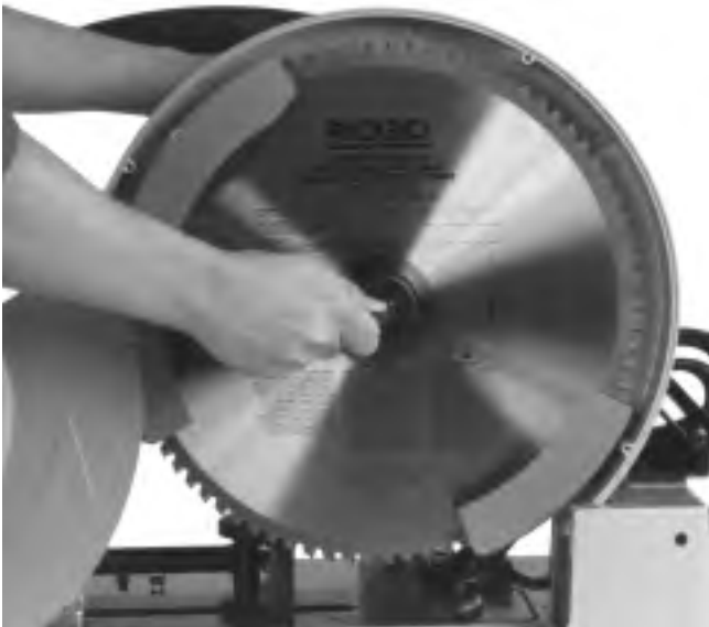
Figure 9 – Installing Saw Blade
