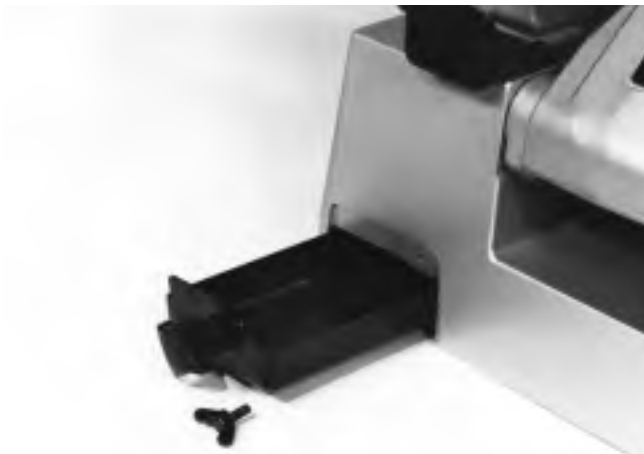
Figure 1 – Cleaning Metal Shavings From Chip Tray
