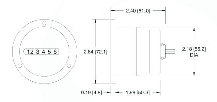
Mounting holes: For #4 screws on 2.44" [62.0] B.C. and #6 screws pm 2.53" [64.3] B.C. Panel cutout: 2.21" [56.1] Dia.
