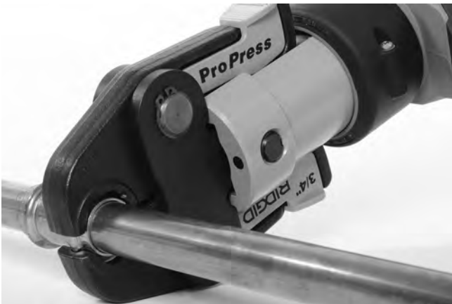
Figure 9 – Placing Scissor-Style Jaws Around Fitting
