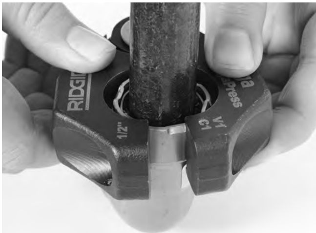
Figure 11 – Installing Press Ring Onto Fitting
