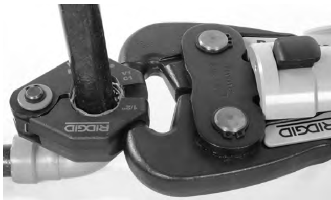
Figure 12 – Attaching Actuator to Press Ring
