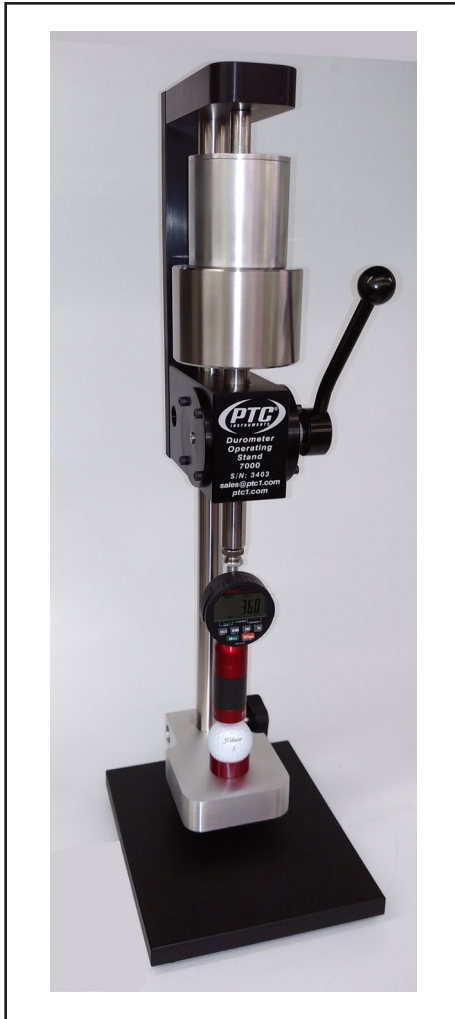
Hydraulic Operating Test Stand #7000D
