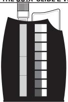
The Octa-Slide 2 Viewer should be held so non-direct light enters through the back of the Viewer. Slide the Octa-Slide 2 Bar into the Viewer. Insert the reacted sample into the top of the Viewer. Match the color of the reaction to the color standards.
