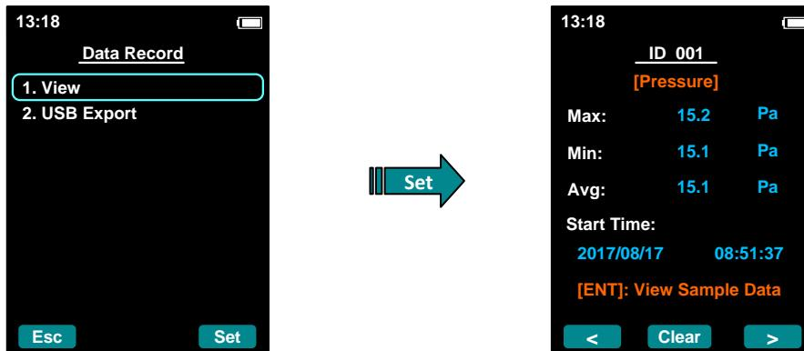
Click “<” or “>” for reviewing the statistic value of differential pressure, air velocity and airflow.
