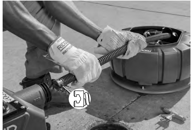
Figure 7 – Inserting Cable Into Front Of Machine
