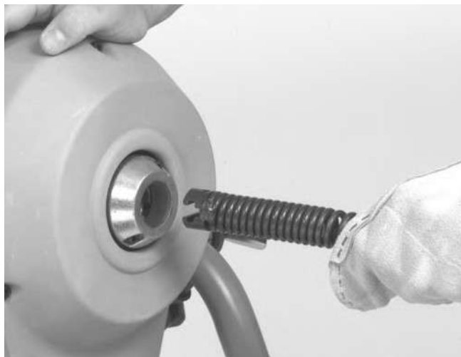
Figure 4 – Inserting Cable Into Front Of Machine
