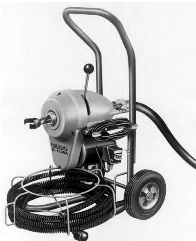
Figure 11 – Storing Cables On “A” Frame Models
