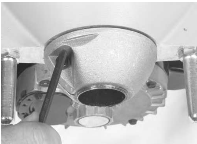
Figure 14 – Removing Clutch End Play
