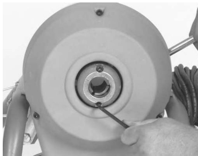
Figure 12 – Replacing Clutch Jaws
