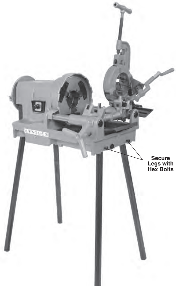
Figure 4 – Threading Machine Mounted On Pipe Legs
