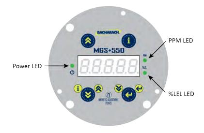
After the warm-up period, the instrument begins normal operation. The display toggles between the current gas concentration and target gas name.
