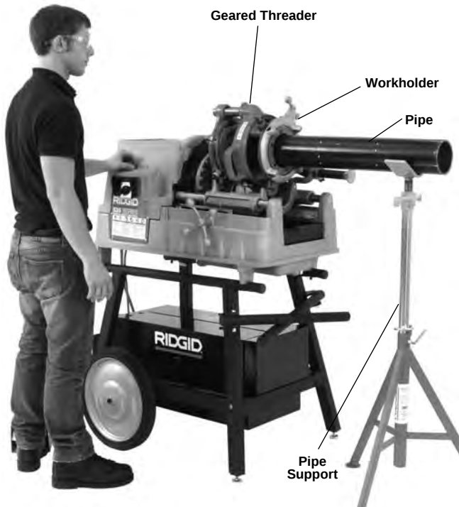
Figure 21 – Operating Position (Close-Coupled Method)
