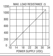
The **SERIES 651** Temperature Transmitters are designed for use with 2 or 3 wire Pt100 RTDs or ungrounded Type K thermocouples. Thermocouple models 651TC are cold junction compensated, automatic 32 to 160°F (0 to 70°C) with upscale burnout.
