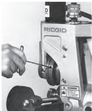
Figure 11 – Loosen Set Screw in Groove Roll
