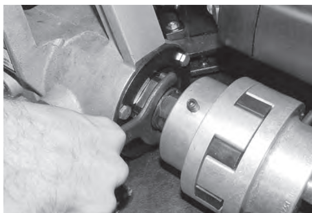
Figure 14 – Loosen and Remove Drive Shaft Retaining Nut
