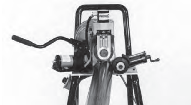
Figure 7 – Offset Pipe on 918-I (exaggerated for clarity)
