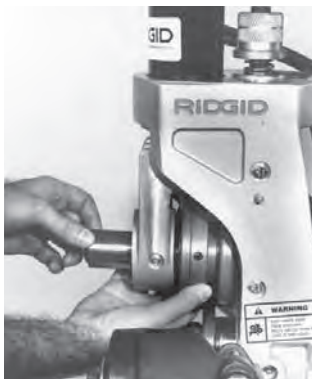
Figure 12 – Remove Groove Roll Shaft and Groove Roll
