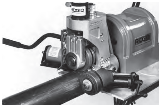
Figure 10 – Adjusting Pipe Stabilizer
