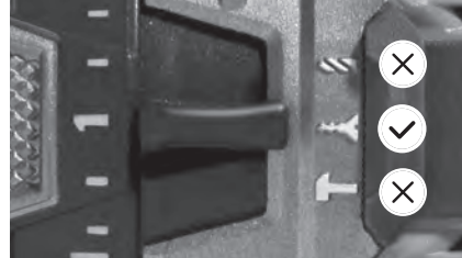
Figure 7 – Selecting Proper Mode
