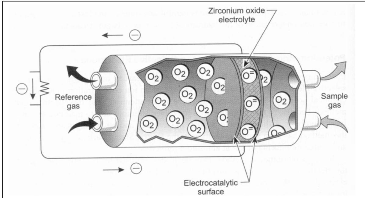
The electro-motive force (emf) that is generated across the solid electrolyte by the presence of oxygen ions can be measured as a sensor voltage (according to Nernst law).
