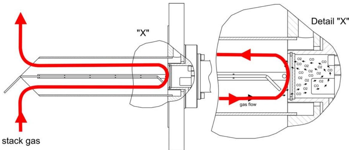
The tube is divided in half by a metal plate welded into the middle of the tube.
