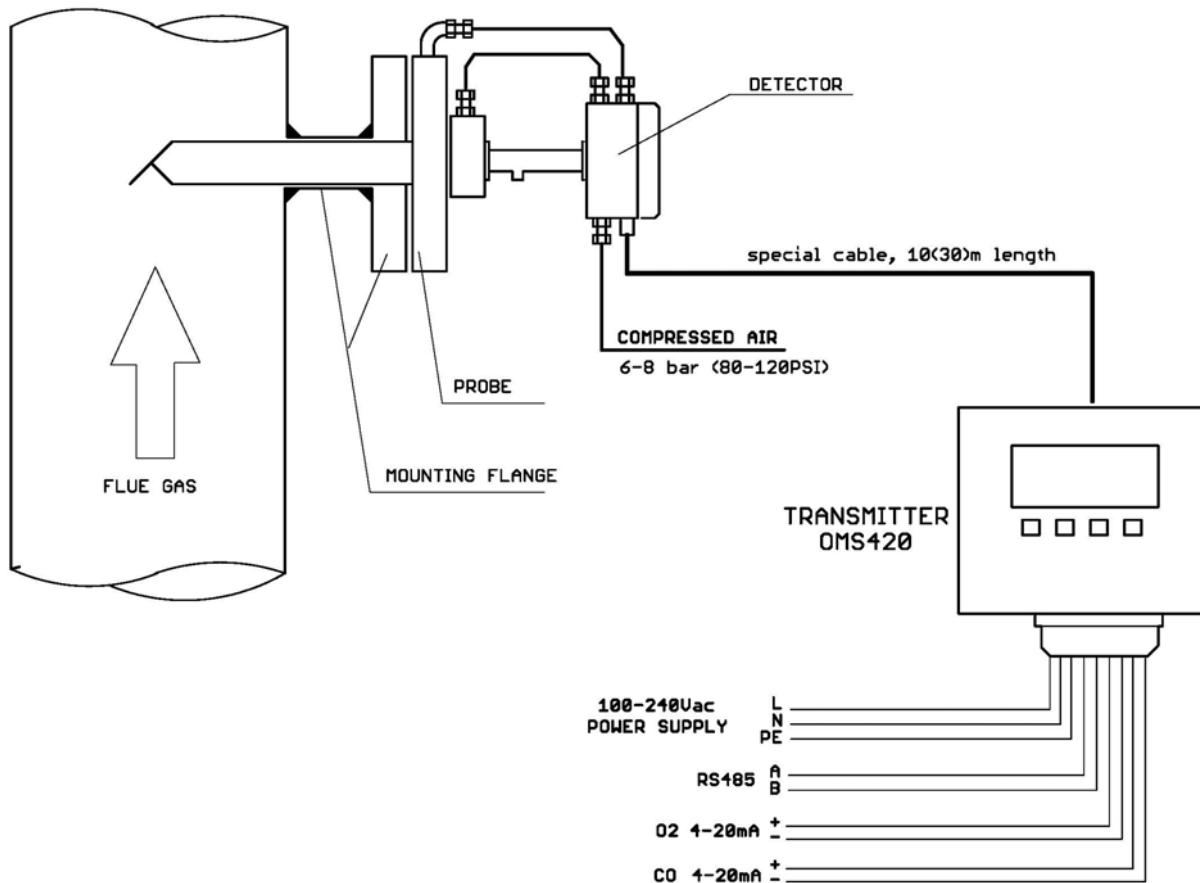
Remote transmitter model components are:
