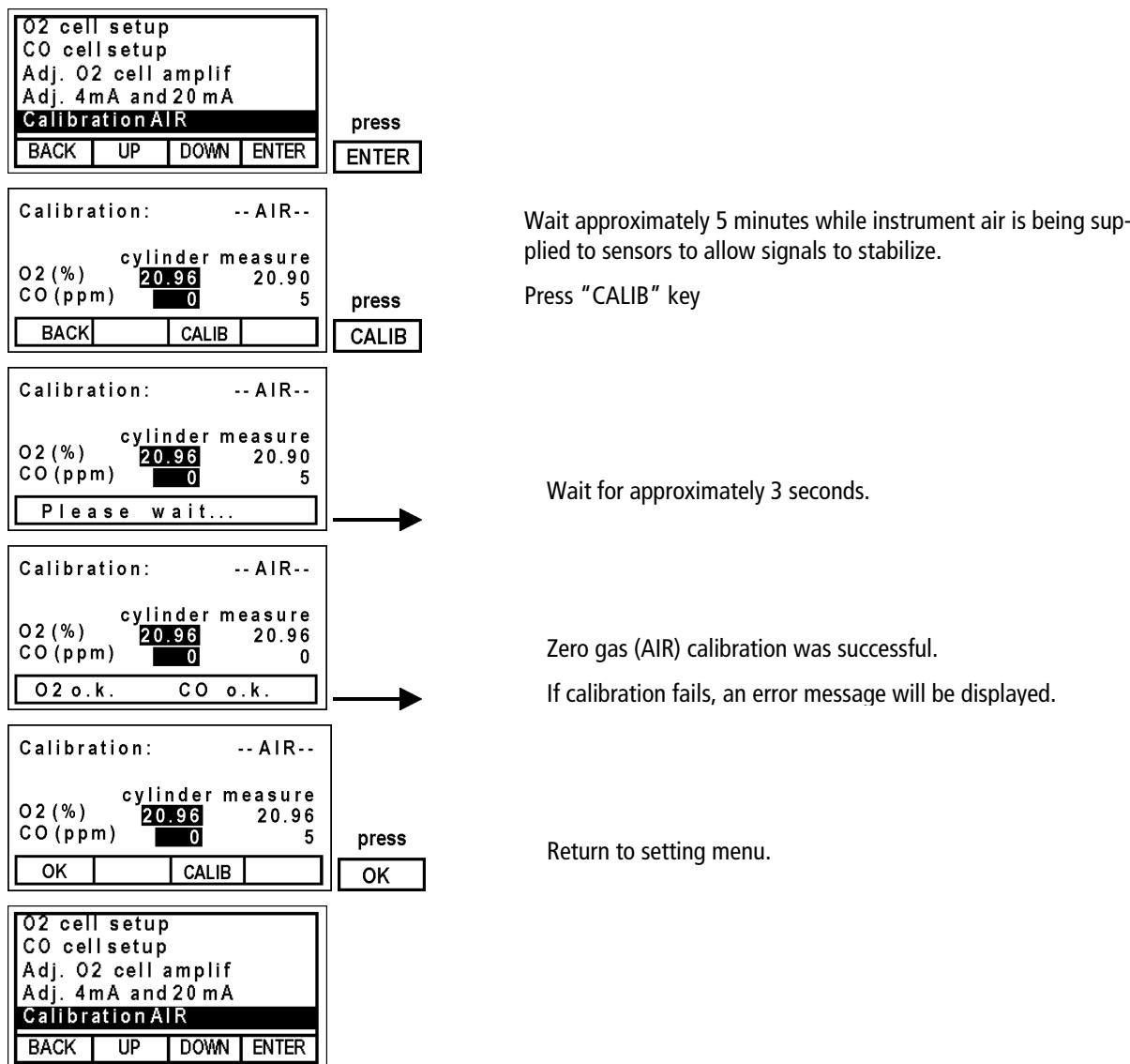
**O<sub>2</sub> OK. CO OK or O<sub>2</sub> failed! CO failed!**
