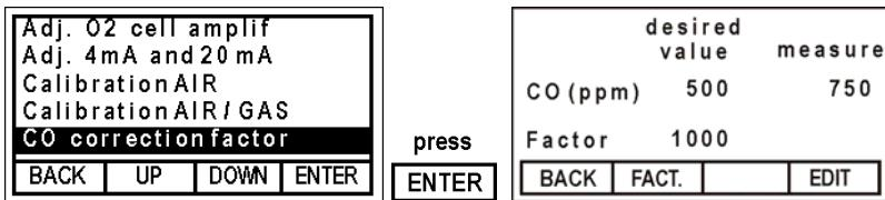
Because sensor is measuring all combustibles in the flue gas, a difference to selective CO measurement will occur.
