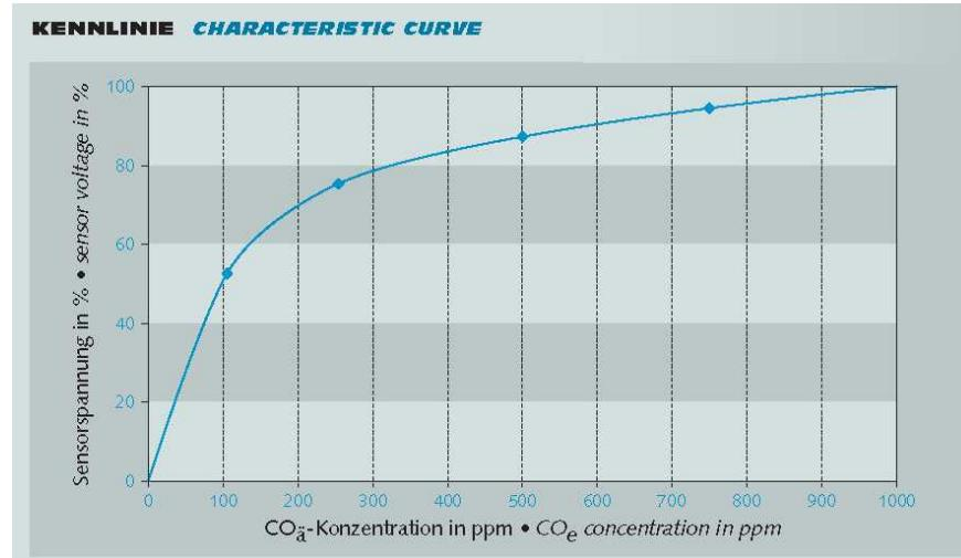
The cell voltage is measured by micro-controller based transmitter electronics and converted into a standard, linearized 4 – 20 mA signal for combustibles equivalent carbon monoxide (COe) in the range of approximate 0 – 1000 ppm.
