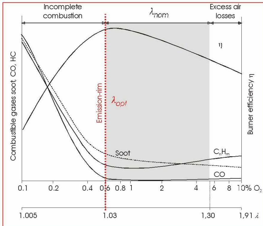
The absolute value of combustibles in the stack gas of a burner depends very much on the design and construction of the burner/boiler. Combustibles (CxHy) are lower in a well-designed system than they are in one that is poorly designed.
