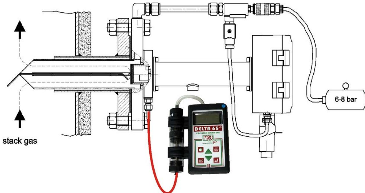
Use a portable analyzer to measure CO in the flue gas and to adjust accordingly the "desired value".
