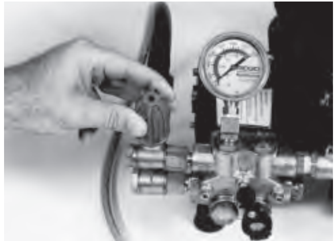
Figure 4 – Adjust the unloading valve
